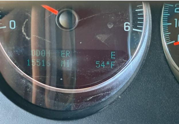
The odometer actually reads over 155K miles; however the last digit does not display.
