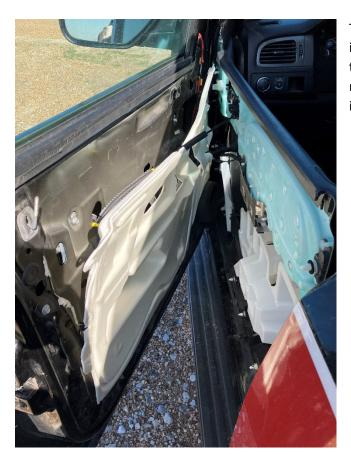
The door has had an issue with the paneling and interior controls separating from the door each time it is opened. Staff have tried different routes to repair this themselves without investing funds on an aged vehicle.
