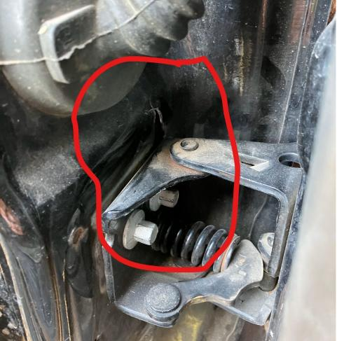
Staff were trying to repair the door facing and found that the internal junction is torn where it meets the door hinge.
