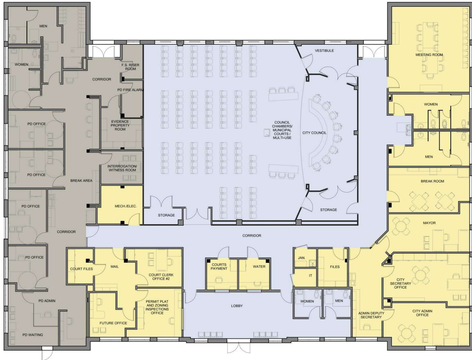
CONCEPTUAL FLOOR PLAN SCALE: 3/16" = 1'-0" JUNE 10, 2020 MUNICIPAL COMPLEX RHOME, TX
