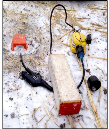
Geophone on the far left, Battery in the middle and Recording Box on right.
