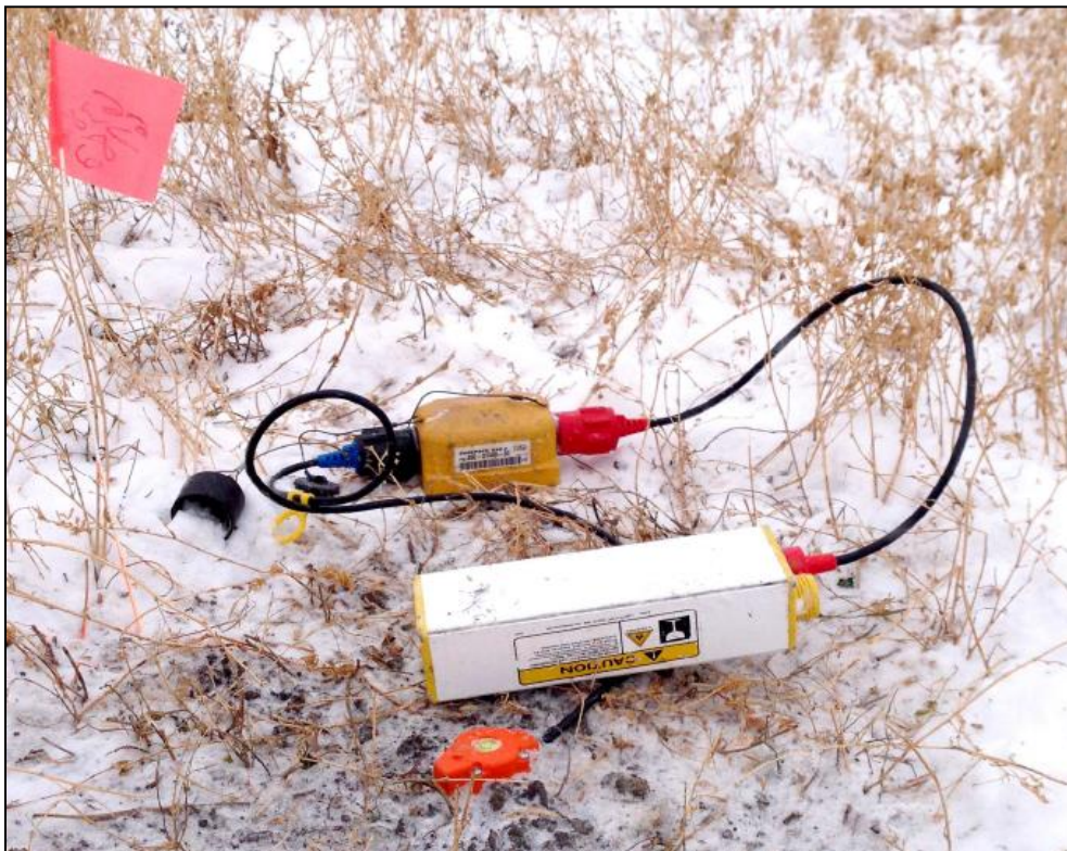
A typical Recording Box, Battery and Geophone on the ground.
