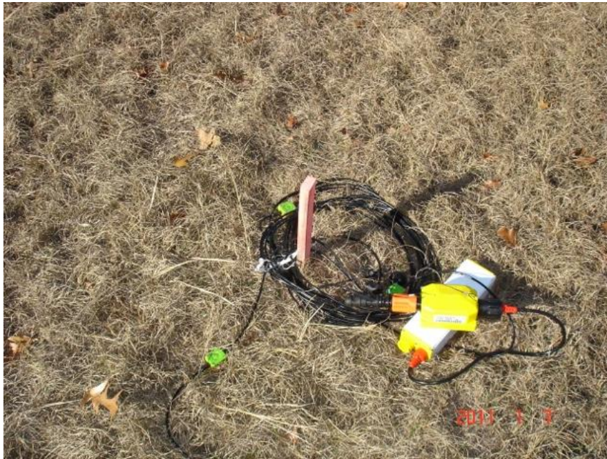
A typical Recording Box, Battery and Geophone on the ground.
