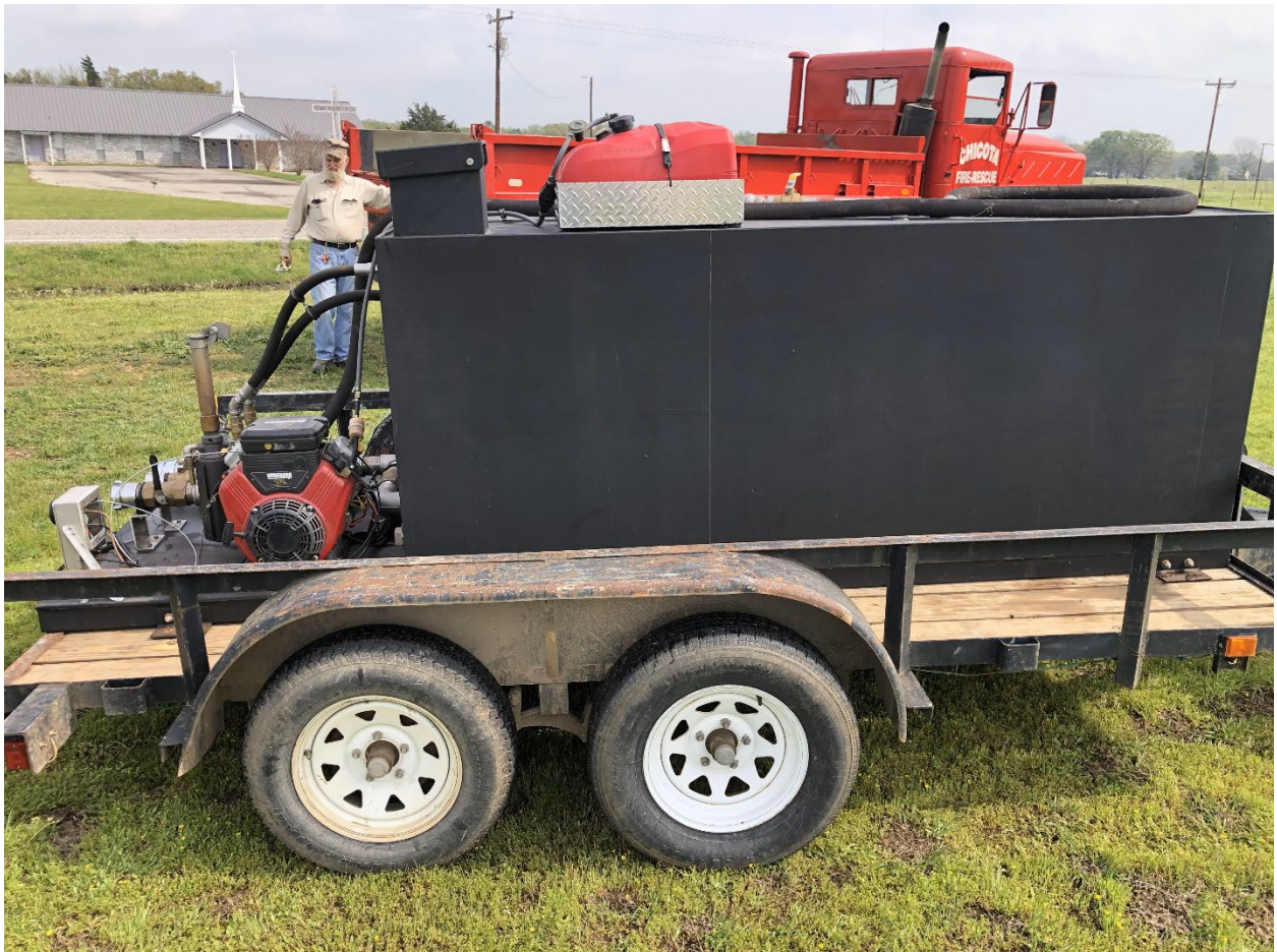
Chicota Skid Unit that would be mounted on our incoming large chassis truck bed
