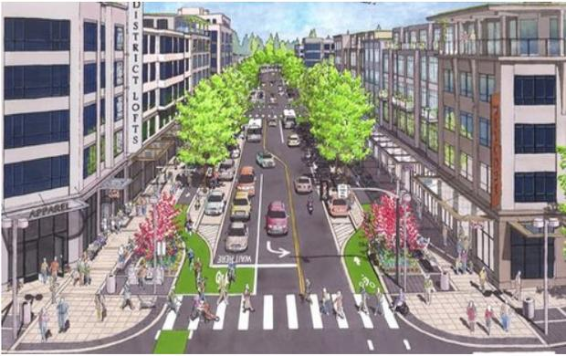
Figure 11-3. A Complete Street design with designated spaces for bike, cars, pedestrians, and transit (Source: Crandall Arambula)
