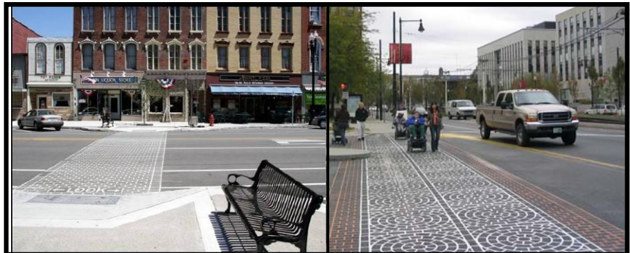
Enhanced Crosswalks: Curb extensions were used in Medina, NY ( left ) in conjunction with a hashed crosswalk to improve the visibility of designated crossing areas on the Village’s historic Main St. (NYS Rt. 63). In Boston, MA ( right ), a neighborhood association worked with the State DOT to choose a unique decorative printed crosswalk.
