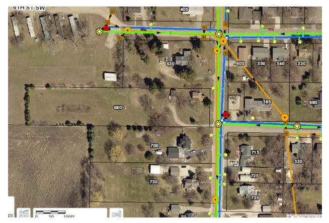
Note: Blue is Water, Green is Sewer, Orange is Storm Sewer
